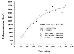
Fig. 2. Build-up of radon in the accumulator chamber
