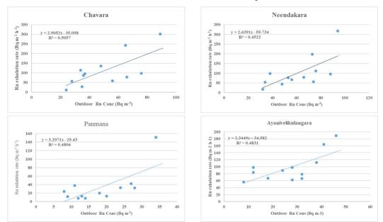
Fig. 4. Relationship of radon exhalation rates from soil with outdoor radon concentration in the four villages
