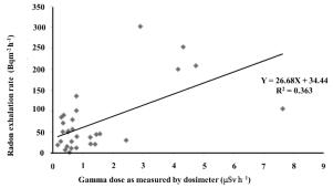
Fig. 3. Scatter diagram of radon exhalation rate against gamma dose in beach regions (Chavara and Neendakara)
